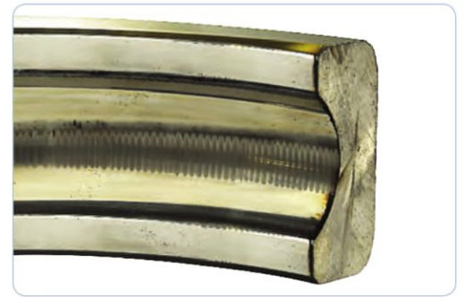
Bearing fluting, "washboard" pattern on bearing race
