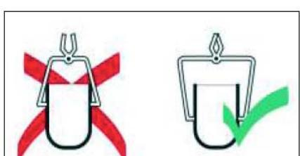
Lift-out tongs should hold crucible on its lower third and fit evenly on both sides.
