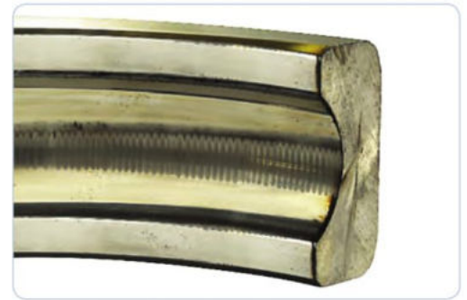
Bearing fluting, "washboard" pattern on bearing race
